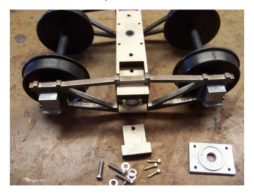
Tilt the bolster leaving the spring plank flat and the springs should pop out. You may need to pull them out. Now tilt both the bolster and spring plank so they are both 90 degrees from the flat position. This will allow you to slide the side frame off allowing the trucks to fully come apart. There are thin, white nylon washers on the axle tips so don't lose them. I added them in case you plan on running the car on electrified track.
