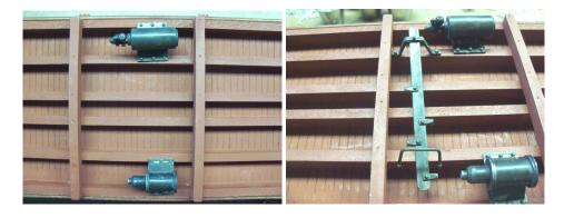
Position the secondary brake lever support as pictured. Drill into the needle beam and sill with a #56 bit and pin with NB's. Slip the brake lever in place and pin with an NB. Measure the distance between holes in the rear of the cylinder and reservoir. Add 1" to this and cut a piece of blackened brass wire. Bend up ½" at each end and then bend out ¼". Adjust the angles of the bends to fit into the rear of the 2 holes and glue in.
