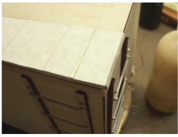
The second row of tiles is all the shorter tiles. The tiles are staggered by 50% so start the first tile as pictured. Only the first and last tile will have an edge bent.
