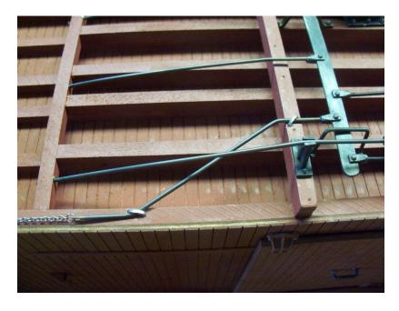
Now glue the 4 bolster reinforcing boxes to the edges of the body bolsters. Drill a #56 hole through the holes and pin with 2 NB's. The NB's will help keep the blocks attached.
