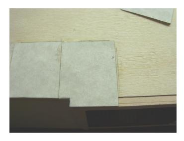
Over the door, the tiles just get a little bending to fit the contour. Trim to fit the last tile over the door and then shift back to the shorter tiles and continue to the right side of the car.
