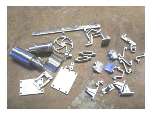
Glue the cylinder saddle to the base (left) and the reservoir saddle to the base (right). Then glue the cylinder to the saddle (bottom) and the reservoir to the saddle (top).
