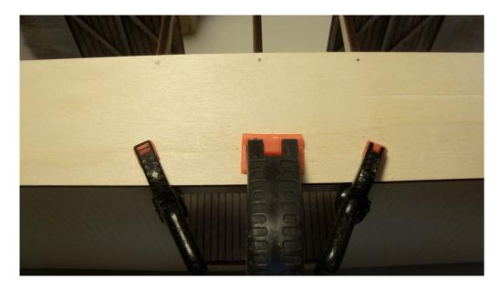
First half glued and nailed. Don't nail the side edge of the 3 center rafters at the door as the brad will come through and draw blood from someone reaching into the car. Just clamp and let dry.
