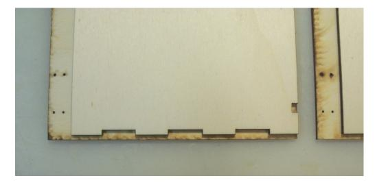
The tabs in the ends are reversed from these tabs and will glue into them creating a strong joint. Do this gluing job on a super flat surface. I have old worn out spin casting molds that I use for weights to firmly press the outer and inner sides together. This is very important so that the end joints will fit together properly.
