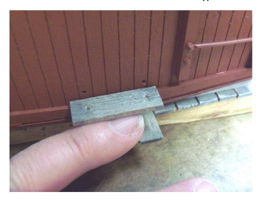
Mark the board to match the holes in the car end. Drill these 2 holes with a #52 drill bit.
