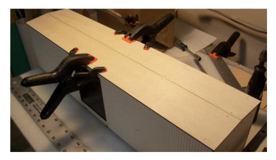
Now mark for brads, the second roof half, add glue and nail to the car. Again, just clamp at the doors.
