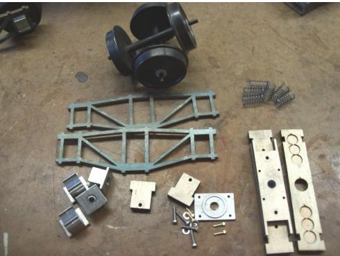
Take the sideframes outside and rattle can them with flat black paint. I sprayed them on a piece of cardboard and then worked on staining with India ink and alcohol all the wood parts. I also shined up the white metal and diecast journal boxes and blackened them with patina. When dry, I buffed the blackened parts with a wool wheel in my Dremel. By this time, the first side of the sideframes were dry and I flipped them over and sprayed the other sides.
