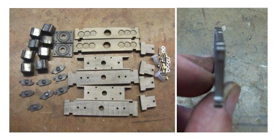
If you hold up a sideframe and look down its length, you'll see it is slightly warped. This is from the heat of the laser cutting them from a large sheet of 11 gauge steel. When you re-assemble the trucks, you want the middle bowed out from the truck. If you reverse them so the journal box ends are bowed out, the wheels and journal boxes will be overly loose and sloppy.
