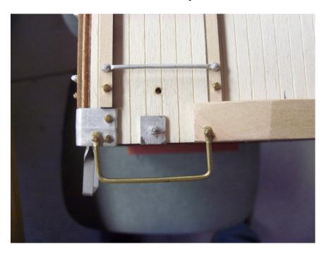
Hold the other brass strap over the buffer and drill a #56 hole into the top of the buffer as pictured and pin with an NB. Holding the strap in position, drill a #56 hole into the car end and pin with an NB.
