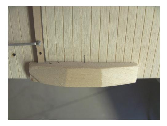
Glue and clamp the buffer to the end of the car and test fit the ladder. You will probably have to sand the bottoms of the legs so when glued, the rungs on this and the side ladder are equal height. Again, be aware of the mounting hole positions. Only the top 2 holes are above the rungs. Drill the 6 mounting holes with a #56 bit and pin with 6 NB's.
