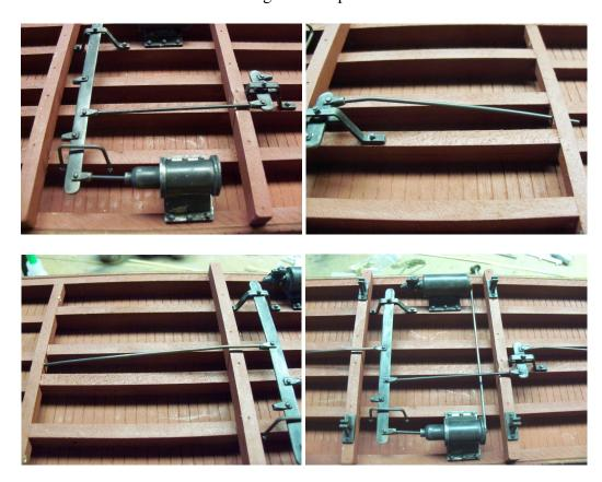
Push one the truss rods into the hole in the truss rod terminating block, bending over a queen post, through a turnbuckle, over the next queen post and down into the hole in the truss rod terminating block. Do the second truss rod the same way.
