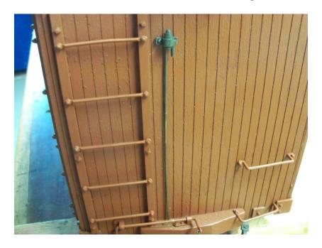
Insert the 1/16" by 8" piece of music wire in the buffer and glue a piece of left over fascia board centered around the wire. Place the upper brake staff support over the wire and rock it enough to mark this piece of wood.
