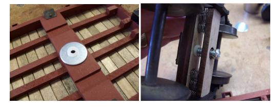
If the screw is working loose during operation, try a little silicon on a tiny portion of the screw threads. When silicon is dry, it's doesn't dry hard but remains flexible so you can remove the screw and trucks at a later point for maintenance.
