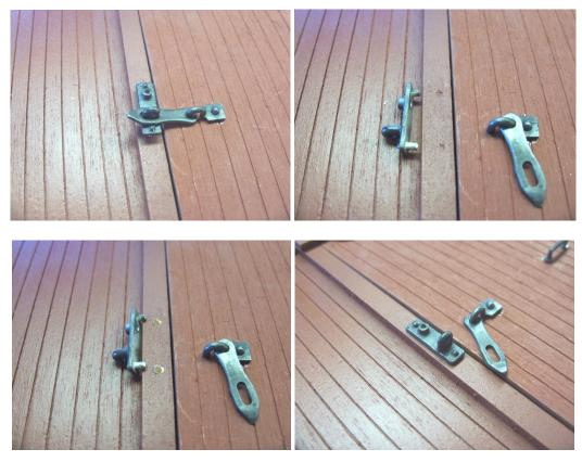
Drill a #56 hole through the hole in the latch plate through the wood door trim and the car side. Press the rivet through the lock pin and into the hole in the plate. Press it down snug but not tight. This will allow the locking pin to move to lock the latching bar to the plate.
