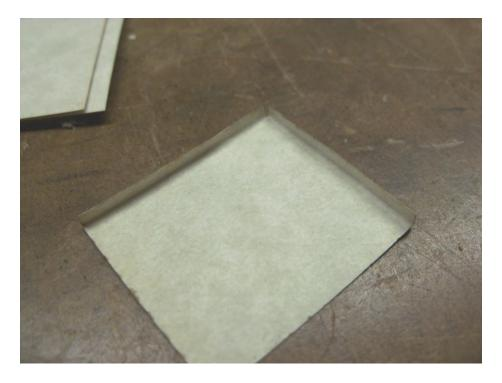
Lay this first tile on the lower left corner and mark its edges with a pencil.
