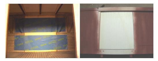
Spray this side of the car. When dry, remove the two cut outs and tape into the other side and paint it.
