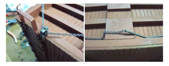
Push the rod back into the third clevis. If too much slack in the chain, remove and trim a tiny bit from the clevis end of the rod and retry. Trim as necessary until the chain is snug with the rod fully inserted in the clevis. Now press the staples into the needle beam and side sill enough to make a mark. Drill with a #56 bit and press the staples in. Add glue to the clevis and staples.
