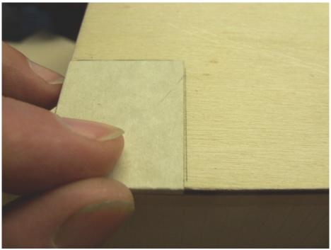
Remove the tile and apply a little glue. I use my index finger to spread the glue evenly and press the tile down. I keep a little bowl of water and paper towels to clean my finger after every 10 or so tiles.
