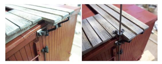
Glue the brake wheel to the top of the staff and slip through the lock pawl, upper support and into the buffer. I don't glue mine in to make transporting less likely to bend or damage any of these parts.
