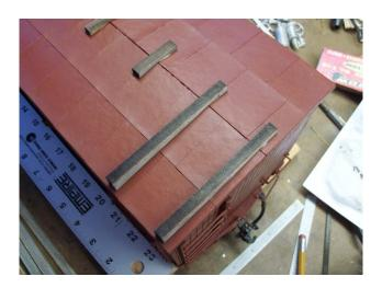
When I want grain on any stick wood, I put a cheap Harbor Freight wire wheel in my drill press with a block of wood as a backstop and run the stick wood through it. Then a light stain.
