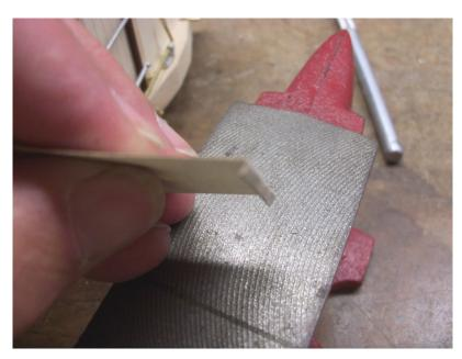
I bend up several at a time, so I don't have to stop gluing to bend. Overlap each tile a 1/16" or so.
