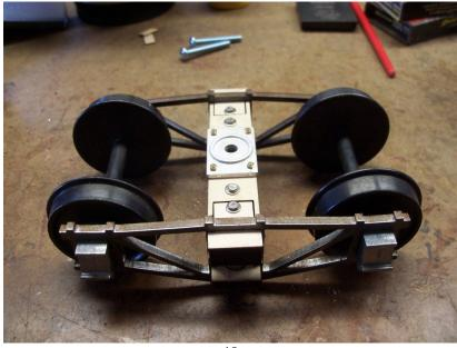
Using a 1/8" socket (3.2mm will work), remove the 4, 2-56 hex head screws and #2 washers. Also remove the 4 NB's and white metal bolster pivot plate. Also pictured is my 1/8" socket wrench.
