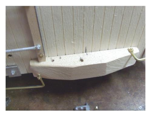
Glue the coupler lift bar in place. Repeat for the other end but you don't have the brake staff or retainer air-line holes.
