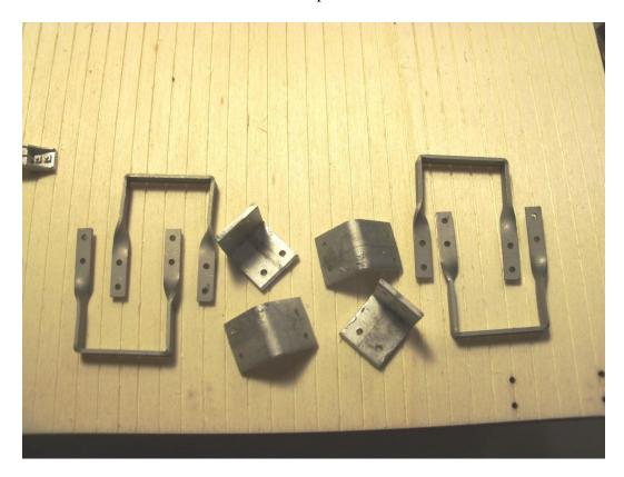
With the car on its side, position 2 of the corner braces on the corners. Drill #56 holes through the 2 holes in the side facing up into the car and pin with NB's. Position a strap step over the 4 lasered holes next to the corner and pin with 4 NB's. Be cognizant of the twist in the side arms of the step so they curve into the step and not out
