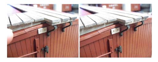
Glue the upper brake staff support into the holes. Slip the brake staff through the support and into the buffer. Slip the lock pawl over the brake staff and position as pictured. Drill one #56 hole through the brace arm and pin with an NB. Drill the remaining 2 holes through the brace and pawl and pin with NB's
