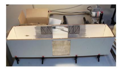
Do this to verify the 4 corners fit together properly. If the floor didn't get positioned 100% over the frame, it might have an edge overhanging the frame on one or more sides. If so, just sand any overhang flush with the sides of the frame. Once you're satisfied with the fit, glue the sides and ends to the frame and to each other. Clean any excess glue from the joints and clamp all sides together to ensure a tight fit in the corners.
