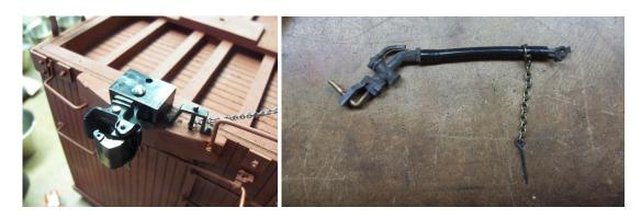
Drill a #52 hole 1-1/4" from the edge of the car into the end beam and a #66 hole in the buffer next to the coupler. Glue the angle cock into the #52 hole and press the eye-pin into the #66 hole. Attach a 3mm jump ring through the coupler chain and through the coupler lift bar hole and close the jump ring. While this won't operate the coupler jaws, it looks good.
