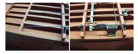
I designed the queen post with deeper than normal slots for the truss rods. This will allow the tops to be slightly bent in with pliers to hold the truss rods from popping out the post. This is white metal and can brake if too much pressure is applied. Just squeeze the tops a little to hold the rods in place.
