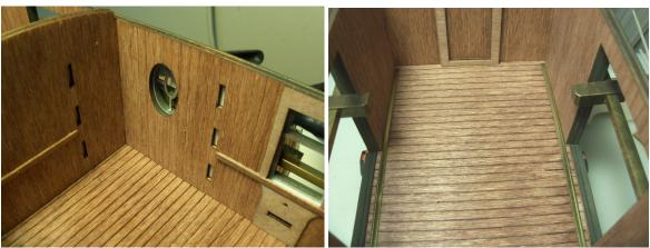
The larger brass clamps easily fit between the car ends and the baggage door openings and the upper windows you left the glass out of.
