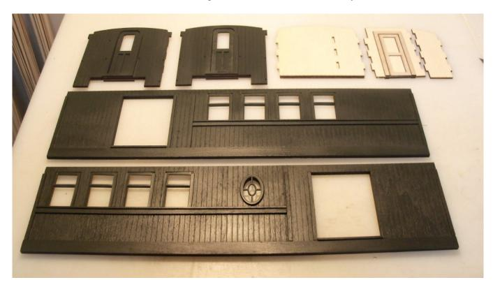
When dry, add all the window panels and chair rail to the inside of the walls. Also add the bathroom door as you did with the coach bath walls. Chair rail will only be applied to the coach end of the car. When dry, stain all the inner walls.
