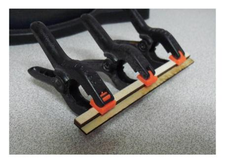
When dry, stain the birch plywood side and glue to the inside of the baggage section with the baggage door set into the brass channel. The glide should be even with the top of the side walls. Make sure the door can slide back and forth and no glue gets into the space where the door slides. Clamp until dry.
