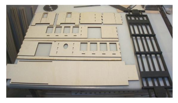
As emphasized in the coach instructions, all these walls need to be glued together flat, aligned and snugly together. Use plenty of weight to squeeze the walls together. Here I'm using old spin casting molds.
