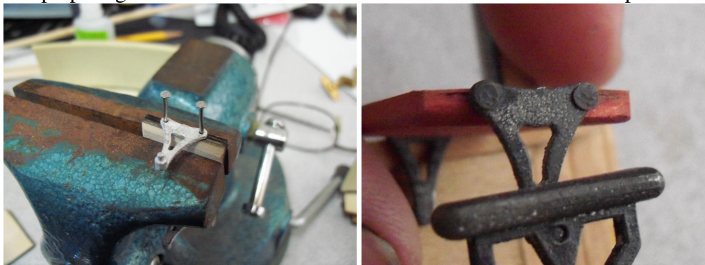
Drilling and preparing to nail the arm to the seat back. Rocker and back are unpainted for clarity.
