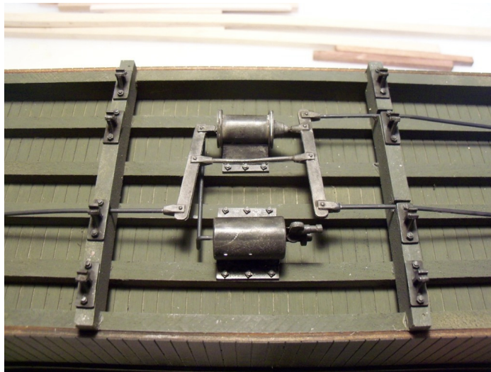
Queen post glued in place in the left picture. Truss rods and turnbuckles added right picture.
